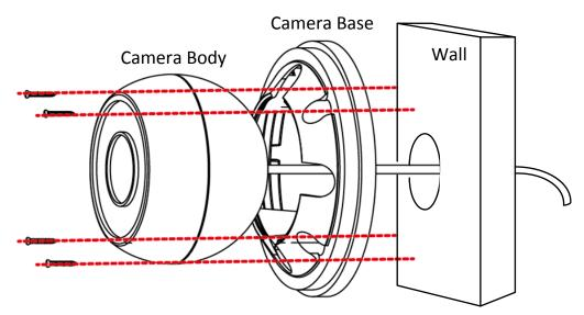
4. Screw back the **Outer Housing** and adjust the camera angle simultaneously.
