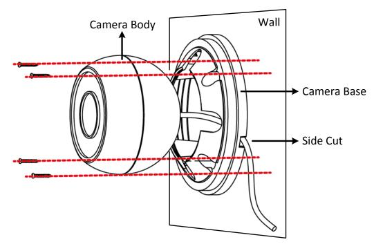
b. If you want to wire the cables through the surface:Attach and screw the Camera Base to the surface with the supplied 4 Screws, and then attach the Camera Body to the Camera Base.
