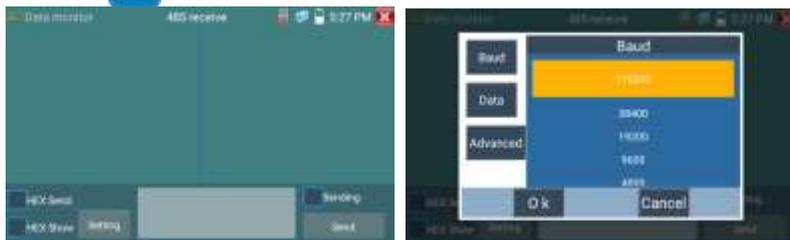
Click "Setting" to choose the baud rate of RS485/RS232; it must be the same as the DVR or the Control keyboard. The DVR or Control keyboard send the code to the tester, if it can be read, the protocol will be shown on the upper right, like Pelco D, if not, like P:---
