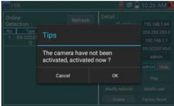
**2. Input password:** Input new password, tap “ok” to activate
