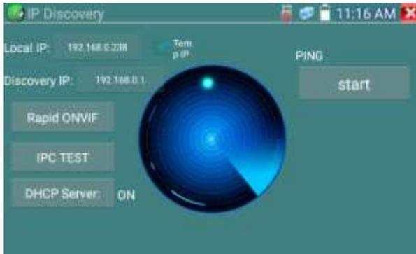
**Local IP:** Tester's IP address, Tester can auto-modify the tester's IP to the same network segment with the scanned camera's IP
