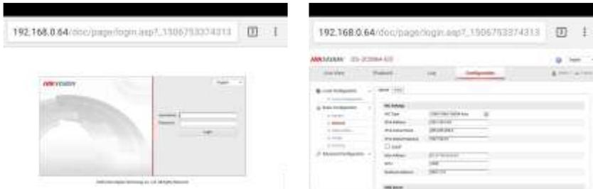
The IP camera and IP tester be on the same network segment for the browser to interface with the camera. If they are not in the same segment, press "RETRUN" to exit. Open the "Settings" app from the main menu to change the IP tester's network settings to match those of the IP camera.
