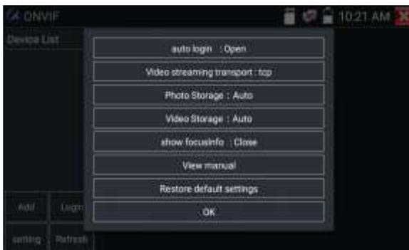
**Auto Login:** After open this function, tester can auto login camera and display camera image (The login password is the same with last time, the first time using password is the default password "admin")
