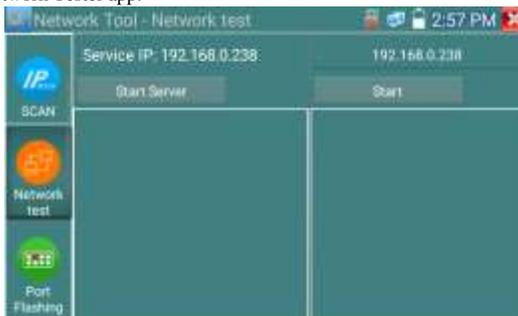
a).**Start the server:** Click “Start Server” button to use the tester as a Server. It will display its IP address at the top of the screen.
