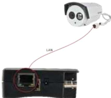
**Note:** If the IP camera requires PoE power, then connect the IP camera to the IP tester's LAN port. The tester will supply PoE Power for the IP camera. Click on the icon labeled POE to turn the PoE Power off or on.
