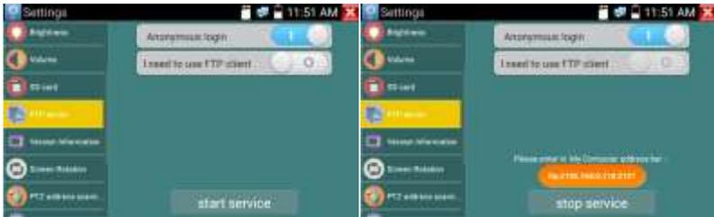
Start the FTP server and then input the tester’s FTP address in the PC’s address bar. This will enable the PC to read, copy and edit the files from the SD card without the use of SD card reader.
