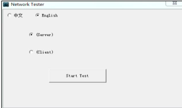
Tester as Client, tester's IP address is:192.168.0.238. The Server and the Client are at the same network segment, but with different IP address. Input Server's IP address 192.168.0.237 in the tester and click "Start" to test network bandwidth.
