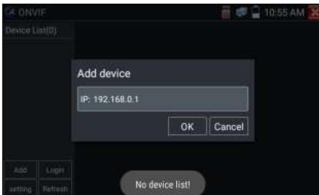
Click the button “Refresh”, tester will scan the ONVIF camera again. Click the newly displayed ONVIF camera on the “Device List”. The tester will show the IP camera’s relative information and settings.
