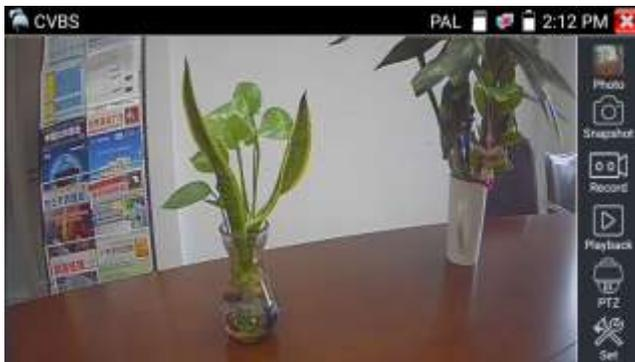
Select relative function on the right side Toolbar to operate , functions including “Photos”, “Snapshot”, “Record”, “Playback”, “PTZ”, “Set”,
