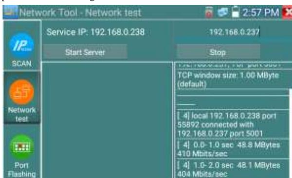
Network bandwidth testing can also be tested with a computer using compatible network bandwidth testing software. Install network bandwidth testing software on a computer, as a test Client or Server, to do the mutual testing with the tester. If use computer as the server, the computer IP address is :192.168.0.237
