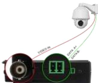
(1) Connect the CVI camera's video output to the IP tester's "Video IN" interface, the image will display on the tester. The tester only come with CVI input interface. There is no CVI output interface.
